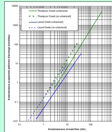
This graph shows the relationship between sediment transport and flow. Lines were fit to a series of individual sediment transport measurements for each gage.
