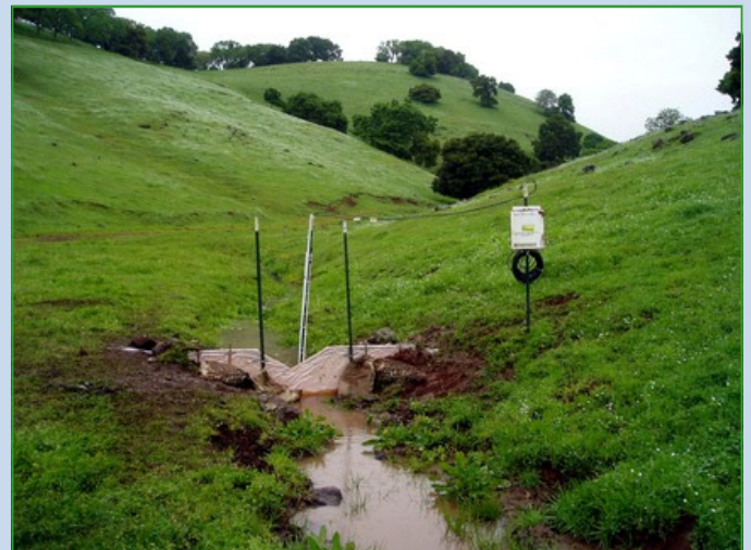
Using stream gaging to calibrate model output.
