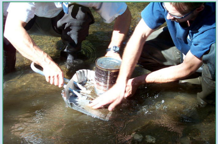
Sampling bulk stream material for analysis
