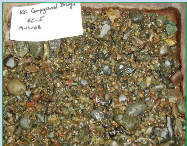
Preparing bulk sediment samples for sieve analysis
